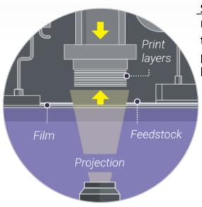
\_Slurry is tape cast onto a transparent film. UV light source projected onto film, curing the resin and forming the 2D slice of the 3D part; process repeated followed by binder burnout and sintering
